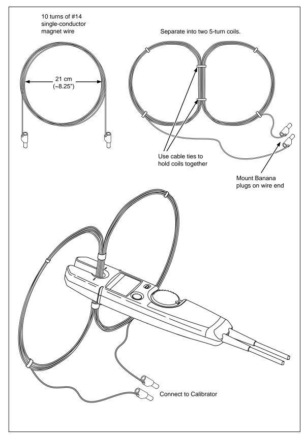
Figure 1. Making the Butterfly Coil
