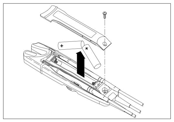
Figure 2. Replacing the Batteries
