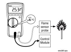
To measure flame rectification circuits:
