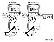
With the function switch in the  $\overline{pv}$ — position, the Meter measures ac plus dc millivolts. Press — to switch the Meter to dc millivolts.
