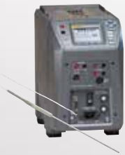
9144 Field Metrology Well and 5615 Secondary Reference Temperature Standard See pg 17
