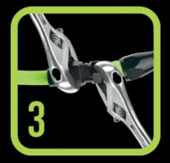
TIGHTEN – Tighten fitting nuts until snug.
