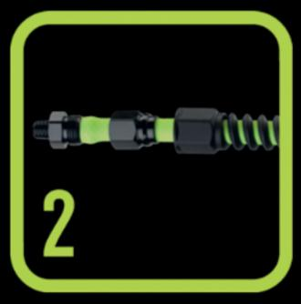
INSTALL – Slide spiral fitting and nut onto hose. Push hose onto fitting until hose reaches threads.
