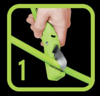
CUT – Measure and cut desired length of hose at 90° angle.
