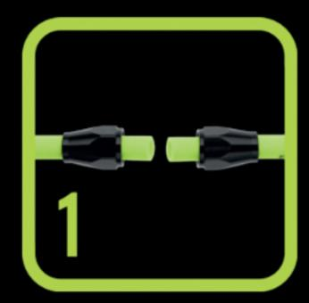
CUT – Cut damaged portion of hose at 90° angle. Slide fitting nuts onto hose.
