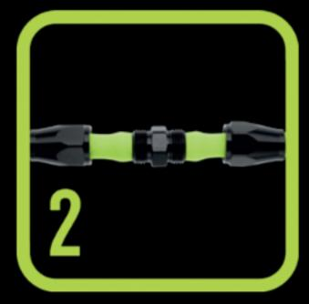
INSTALL – Slide hose onto fitting until hose reaches threads.
