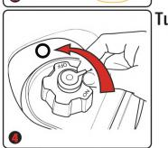
Turn the fuel cap vent lever to the "OFF" (O) position
