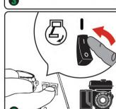
Flip the engine switch to the "ON"(I) position
