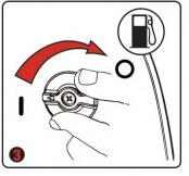
Turn the fuel valve to the "OFF"(O) position
