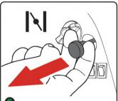
Pull the choke lever out to the "START" position
