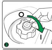
Turn the fuel cap vent lever to the "ON"(I) position
