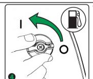
Turn the fuel valve to the "ON"(I) position
