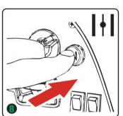
Push the choke lever in to the "RUN" position
