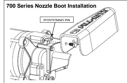
Install the first hole on the positioning pin that is part of the pump end cap casting. Install the attaching bolt in the hole nearest the open end of the nozzle boot.
