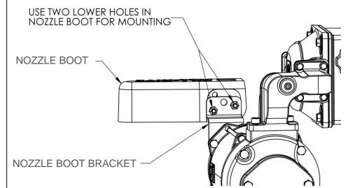
The nozzle boot is installed using the lower two screw holes on the side of the boot. Use supplied attaching hardware to install the nozzle boot.
