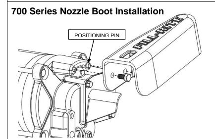
Install the first hole on the positioning pin that is part of the pump end cap casting. Install the attaching bolt in the hole nearest the open end of the nozzle boot.
