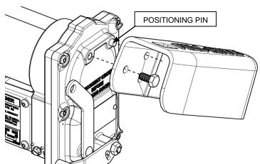
Install the first hole on the positioning pin that is part of the pump end cap casting. Install the attaching bolt in the hole nearest the open end of the nozzle boot. (\*A, B, and C series pumps have no positioning pin: use same holes and 2 bolts to attach boot.)
