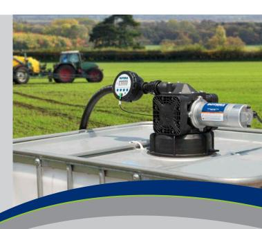
The 800 Series Digital Meter features nutating disc, positive displacement technology. This simple to use, durable meter provides current and cumulative flow totals, and is field programmable for convenience and versatility. It will measure fluids in ounces, pints, quarts, liters, gallons, and in user specified units. The "P" designation in the model number tells you this meter has pulse output, making it an excellent choice for batching, use with FMS and PLC systems, and remote monitoring.
