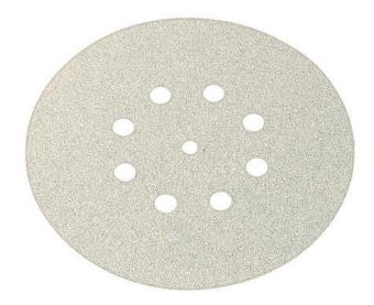
perforated, Ø 150 mm, with hook and loop fastener rapid attachment Application: Metal, car bodies, soldered points, welds, fibreglass. Quality: high-performance emery canvas, fully synthetic-resin bonded, corundum. Features: highly stable, high sanding capacity.
