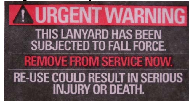
Fig. 10.2 – "Pack-Style" SAL Indicator Label
