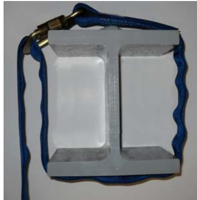
Incorrect Tie-Back Connection
