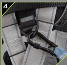
4 Tool Tether connection rings.
