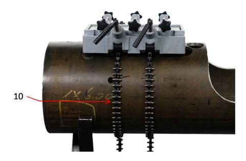
**Step 2.** Hook up the chains (10) into the lock groove, then turn the chain tightening bolt (11) counterclockwise.
