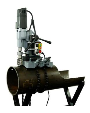
**Step 4**. Turn on the magnet switch and start the motor for drilling work.
