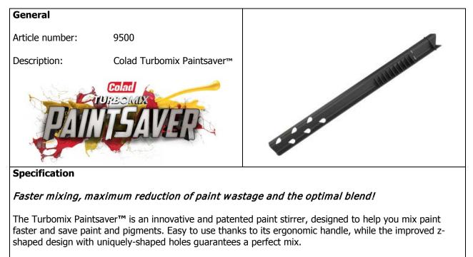
This all results in 30% faster stirring, which increases to almost 40% with metallic paints. The innovative "Break It to Save It" system ensures most paint and pigments are effortlessly removed from the Paintsaver before disposal and it saves time as the stirrer does not leak afterwards. The Turbomix Paintsaver is made from recycled materials.
