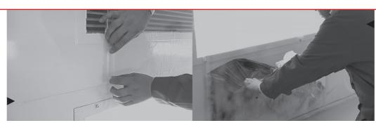
Each transparent anti-static polypropylene layer is treated with paint adhesion to trap overspray.
