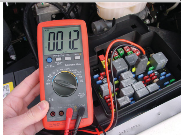
301M Fuse Buddy DMM Adapter in action
