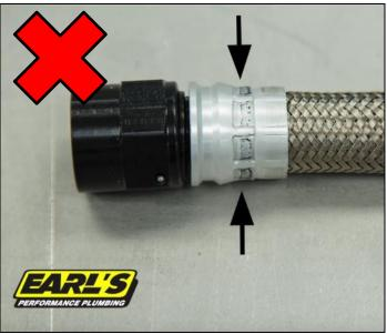
A shallow depth will result in an assembly that is under crimped and will leak.
