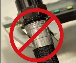
NOTE: If your measured O.D. is larger than the specified range you will need to adjust the micrometer stop and crimp again. If your measured O.D. is more than 0.015" smaller than the specified range then you have over-crimped the collar and will need to discard the assembly and start over.
