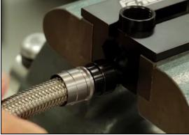
NOTE: ENSURE THAT THE BRAID IS NOT TWISTED OR BUNCHED IN ANY LOCATON AS THIS WILL COMPROMISE THE MAXIMUM PRESSURE HOLDING CAPABILITES OF THE HOSE.
