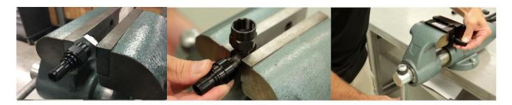
4.2) Next, apply a light coat of Earl's Assembly Lubricant (184004ERL) onto the nipple. Push the hose onto the nipple until the inner liner is fully seated on the step of the nipple. Then, push the collar all the way forward.
