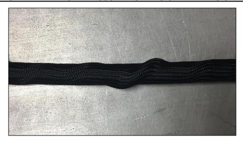
4.3) If the hose liner protrudes past the crimp collar, then you may trim the excess braid being careful not to trim off too much. The key to strength of the Ultra Pro Hose is a tight, straight braid.
