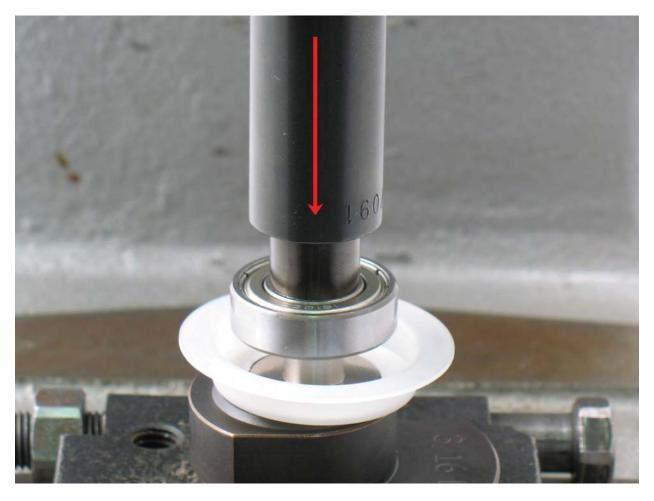
**5.** Use small diameter of **57091** Bearing Press Tool and arbor press to install **58368** Bearing onto motor shaft balancer.
