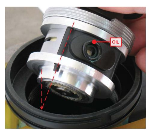
**12.** Apply oil to **01024** O-Ring and install in cylinder sleeve adapter.
