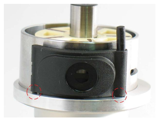
9. Install **59134** Cylinder and **59133** Cylinder Sleeve Adapter so that short pins fit into front bearing plate.
