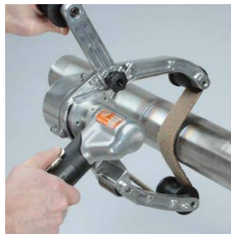
Two-handed use increases operator control.
