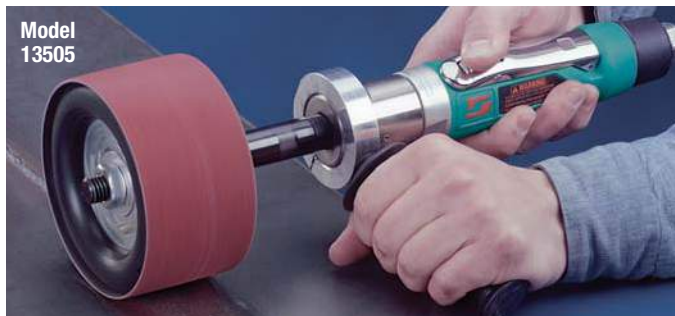
13505 Dynastraight® powers optional 94472 Dynacushion® pneumatic wheel.
