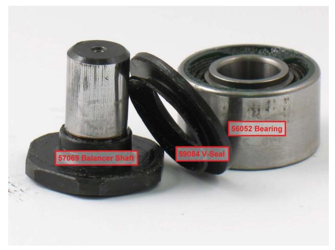
• Remove the **59084** V-Seal. **Motor Disassembly Completed.**
