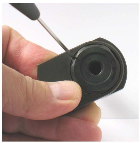
**3.** Compress and install **95630** Snap Ring in groove of motor shaft balancer.
