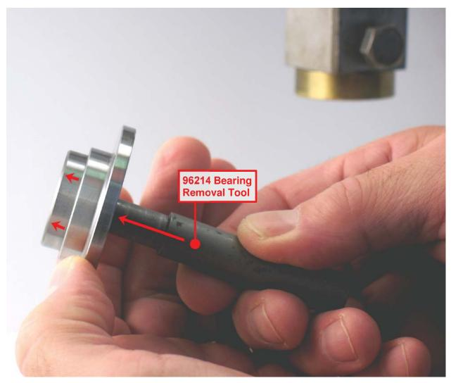
6. By hand, or with arbor press, use 96214 Bearing Removal Tool to remove 58368 Bearing from 59138 Rear Plate.
