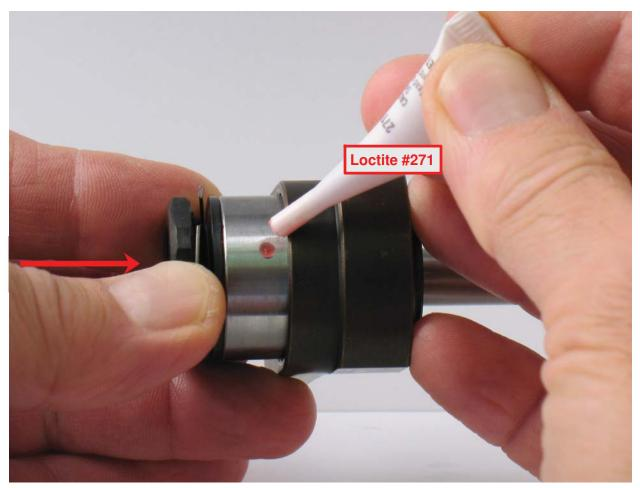
**2.** Apply a small amount of Loctite #271 or equivalent to outside diameter of **56052** Bearing. Install balancer shaft with bearing into motor shaft balancer.
