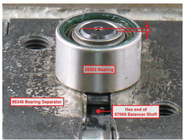
• Fasten bearing separator between **56052** Bearing and hex end of **57069** Balancer Shaft.
