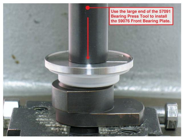
6. Use large diameter end of **57091** Bearing Press Tool, and the arbor press to install **59137** Front Bearing Plate.
