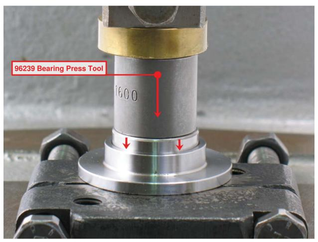
10. Use **RAISED OUTSIDE DIAMETER** of **96239** Bearing Press Tool and arbor press to install **58368** Bearing into **59138** Rear Bearing Plate.
