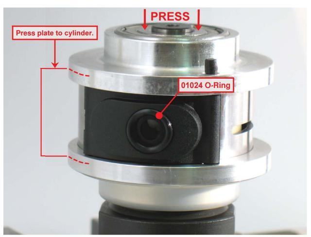
**11.** Use small diameter end of **57091** Bearing Press Tool and arbor press to install bearing and plate onto motor shaft balancer. **Notice:** Carefully press bearing and plate down until it **just touches the cylinder**. This will produce a close fit between the bearing plates and cylinder.
