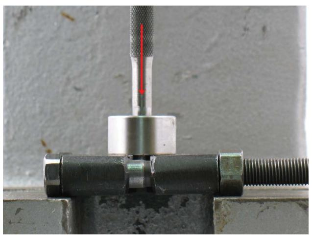
• Use 5/16" or 8 mm diameter flat-end drive punch as press tool to push balancer shaft out of **56052** Bearing.
