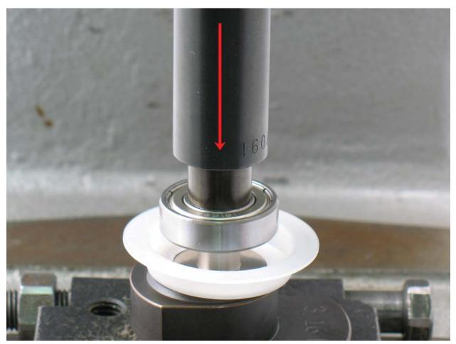
5. Use small diameter of **57091** Bearing Press Tool and arbor press to install **58368** Bearing onto motor shaft balancer.
