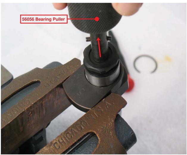
• Use 56056 Bearing Puller to remove balancer shaft and bearing.
