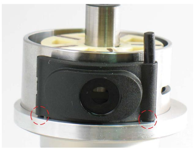
**9.** Install **59134** Cylinder and **59133** Cylinder Sleeve Adapter so that short pins fit into front bearing plate.
