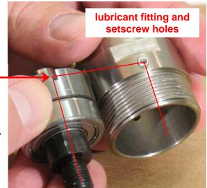
Install the planetary reduction into the adapter and/or planetary housing. Apply Loctite #567 (or equivalent) to the 50784 Setscrew(s) and install.
