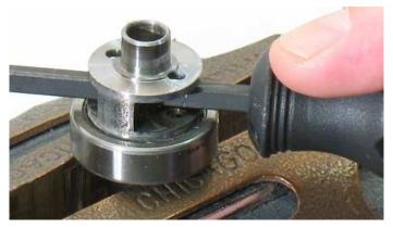
Insert a screwdriver through the carrier and turn counterclockwise to remove the adapter or pinion.
