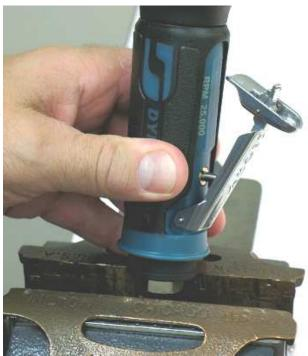
**Notice:** If the **01578** or **94523** Inlet Adapter loosens before the rear exhaust cover or planetary housing, remove the inlet adapter, muffler and valve parts. Fasten the **96399**, 12 mm Hex Key in the vise with the notched end pointing up.
