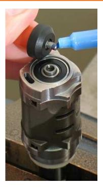
12. Install the 45320 Governor Chamber into the 45305 Housing.
