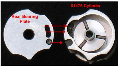
**IMPORTANT:** Carefully press the bearing <u>until the plate just touches the cylinder</u>. Establish a "snug-fit" between the bearing plates and the cylinder.
