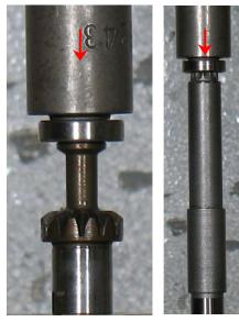
2. Use the **RAISED CENTER** of the 96418 Bearing Press Tool and the arbor press to install the 54537 Bearing onto the 54549 Work Spindle.
