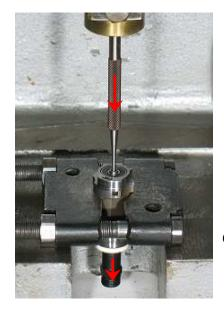
4. Carefully hold the tool spindle or pinion in the vise with aluminum or bronze jaws so that the governor is pointing up.
