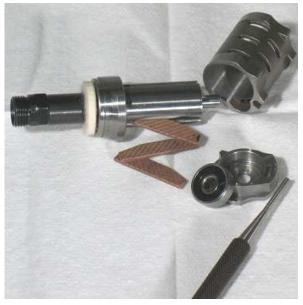
**Notice:** For planetary gear tools, use the arbor press to remove the front bearing and plate.
