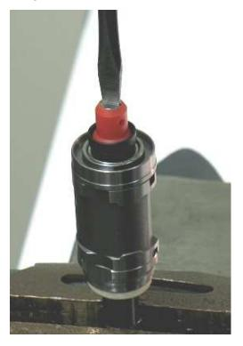
6. Use a 3/32" (2.38 mm) diameter flat-end drive punch as a press tool to push the rotor out of the **02696** Bearing.
