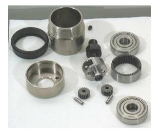
Clean and inspect parts before assembling.
