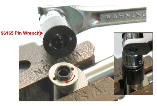
6. Use the 96165 Pin Wrench to remove the bearing cap. LEFT HAND THREAD Turn clockwise.
