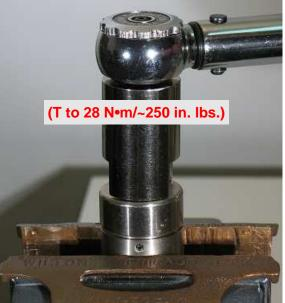
Planetary Assembly Complete.
