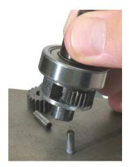
5. Use a 5/16" flat-end drive punch as a press tool to push the planetary carrier out of the "REAR" 54520 Bearing.
