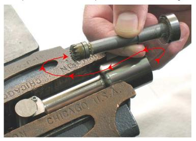
5. Reposition the **54547** Angle Housing and fasten the flat sides of the housing in the vise with the **54550** Bearing Cap facing up.
