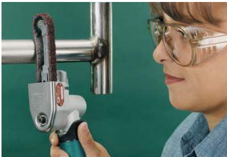
Clean and finish using non-woven nylon belts.
