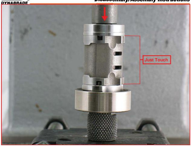
8. Use the **RAISED INSIDE DIAMETER** of the **96242** Bearing Press Tool and the arbor press to install the rear bearing and plate onto the rotor. **Notice:** Carefully press the bearing and plate down until it <u>just touches the cylinder</u>. This will establish a close fit between the bearing plates and the cylinder.
