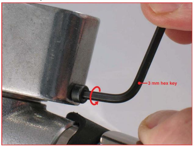
1. Use a 3 mm hex key to loosen the **01788** Motor Lock Screw. Remove the **15060** Housing Assembly from the air motor.
