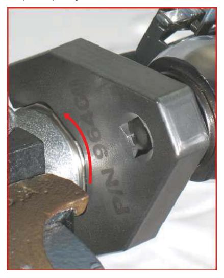
2. Pull the 01558 Collar back onto the throttle body housing. Use the 96460 Wrench to loosen the throttle body from the 7°housing. Left Hand Thread Turn clockwise.
