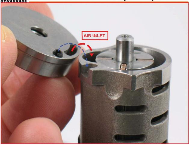
7. Install the **01476** Cylinder so that the air inlet opening in the **02673** Rear Bearing Plate will line up with the air inlet opening of the cylinder.
