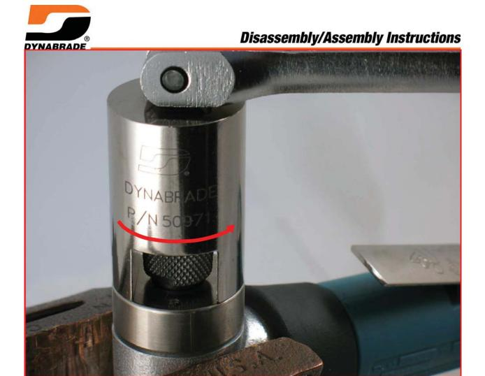
3. Use the **50971** Lock Ring Tool or an adjustable 3 mm pin spanner wrench to remove the **15106** Exhaust Cover. Turn counterclockwise.
