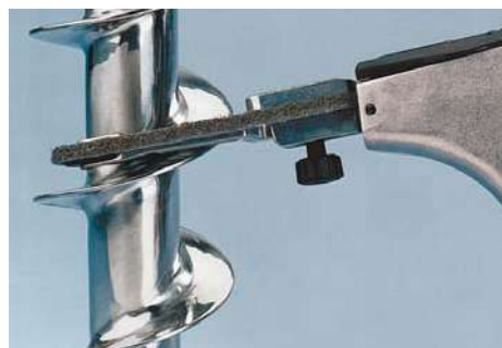
Clean and finish using non-woven nylon belts.
