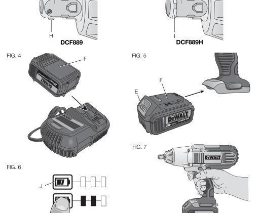
To actuate the fuel gauge, press and hold the fuel gauge button (J). A combination of the three green LED lights will illuminate designating the level of charge left. When the level of charge in the battery is below the usable limit, the fuel gauge will not illuminate and the battery will need to be
