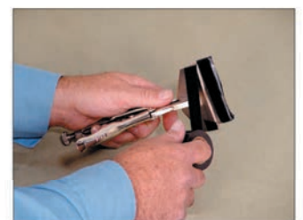
Figure 3 – Any other fit-up clamps should be insulated with tape to prevent unintentional shunting.
