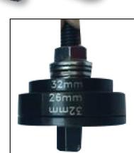
Stack discs on top of each other to create bezels for mounting
