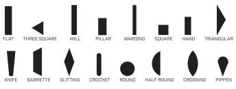
• Area to be filed will determine specific cross-section (round, square, flat, etc.) to be used
