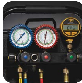
Hard mounted manifolds
