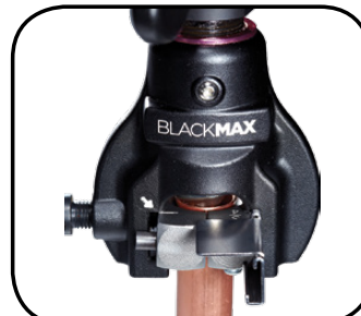
Eccentric flaring cone for precision flares
