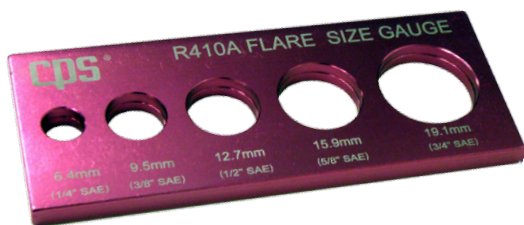
FTXSG R410A FLARE SIZE GAUGE 6.4 mm, 1/4" 9.5 mm, 3/8" 12.7 mm, 1/2" 15.9 mm, 5/8" 19.1 mm, 3/4"
