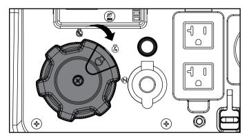
5. Press and hold the yellow ignition switch on the EZ Start Dial toward the center of the dial. Release as the engine begins to start. If the engine fails to start within five seconds, release the switch and wait at least ten seconds before attempting to start the engine again. and hold ignition switch on EZ Start Dial.
