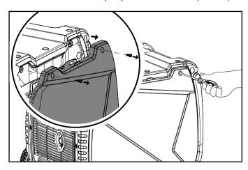
2. Locate the air filter plastic cover and remove by pinching the clips together and pulling the cover off.
