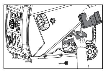
5. Check engine oil level before each use and add as needed.
