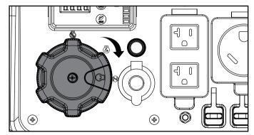
5. Press and hold the yellow ignition switch on the EZ Start Dial toward the center of the dial. Release as the engine begins to start. If the engine fails to start within five seconds, release the switch and wait at least ten seconds before attempting to start the engine again.
