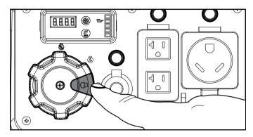
6. Do not over-choke. As soon as engine starts, turn the EZ Start dial to the "RUN" position.
