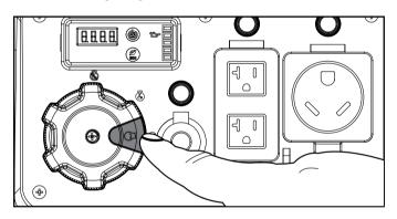
5. Do not over-choke. As soon as engine starts, turn the EZ Start dial to the "RUN" position.
