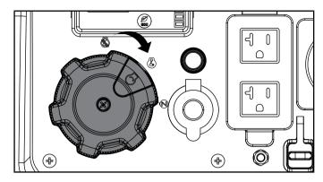
4. Press and hold the yellow ignition switch on the EZ Start Dial toward the center of the dial. Release as the engine begins to start. If the engine fails to start within five seconds, release the switch and wait at least ten seconds before attempting to start the engine again.
