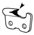
6. Keep all cutters equal. Start with the cutter with the most damage and hand file all cutters back equally.
