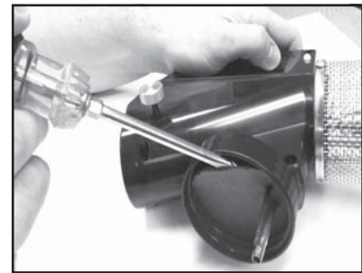
6. Remove and discard gasket from fogger.
