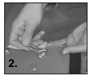
2) Secure spikes tightly using nut and wrench provided.
