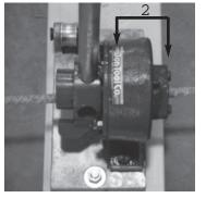
Insert the rebar through the cutting hole in the hub w/bushing to the desired length (add two inches from the back plate (key #4) for actual cutting length).
