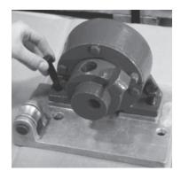
1. Assemble the complete housing unit (key #2) and the base casting (key #3) by inserting the Hex Head Bolts (key #014).
