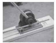
1. Line up the bending arm so that it is in its lowest position (parallel to the roller (key #11)), and then slide the rebar on the roller and into the bending arm.
