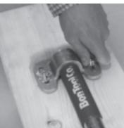
6. For easy storage of Bon's Rebar Cutter/Bender place the steel bar into a socket on the housing unit, and pull the handle down until it hits the board (key #9). Move the handle clip (key #5) over the end of the 54" steel handle and tighten the handle clip down with the 1/4" wing nuts (key #20).
