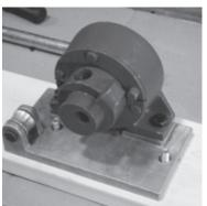
2. Attach the complete housing unit and base casting to the board (key #9) by inserting the 1/2" carriage bolts (key #15) into the bottom of the board. Place the base casting and housing on top of the board and carriage bolts (be sure that neither edge of the base casting is flush with the edge of the board).
