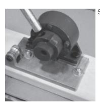
Insert the 54" steel handle (key #8) into one of the sockets on the complete housing unit (key #2) and your unit is ready to use.
