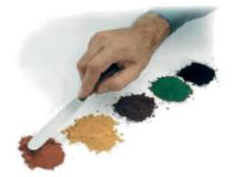
ASTM designation C-979 standard specification for pigments for integrally colored concrete limits the amount of pigments to no more than 10% of the total weight of the cementitious material in the mix.
