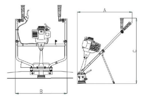
**Hand-Arm vibration** Specification (According to ISO 5394, EN 1033 and EN500-4): 7.8m/s<sub>2</sub>
