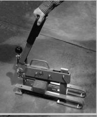
Then, with the handle in the "up" position, place the brick in the center of the blades underneath the Blade Hinge Pin. For accurate angle cutting, use our optional Cutting Guide Table (sold separately).
