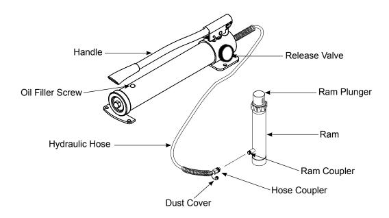
Figure 1 - Pump and Ram Components
