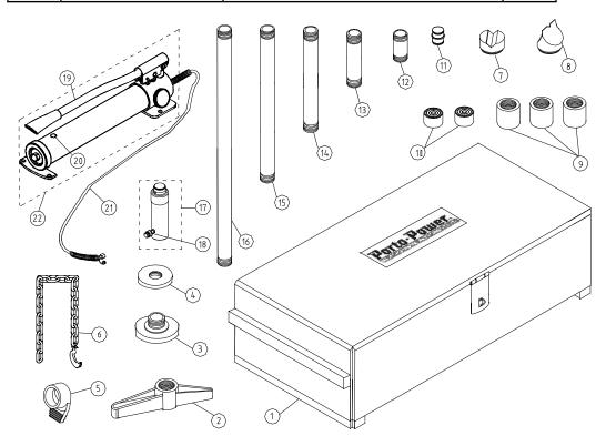
Figure 4 - Replacement Parts Illustration for Model B65041
