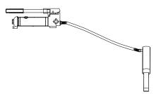
Figure 3 - Illustration to bleed air from system
