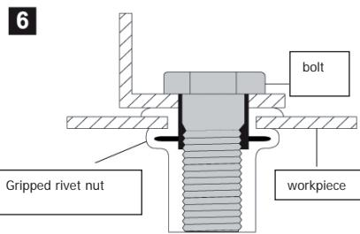
Complete the fastening by fixing a bolt to the gripped rivet nut
