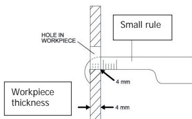
The rule is to measure the Workpiece thickness.
