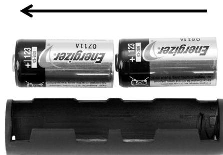
Load two CR-123 Lithium batteries with the positive terminals pointing in the direction of the arrow. NOTE: The flashlight cannot be charged with the CR-123 CARRIER installed.
