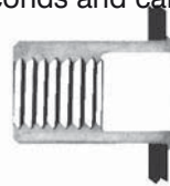
1. Insert TSN into prepared hole.
