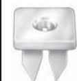
14256 (90189-04014) Natural Nylon #8 Screw Size 10mm Wide, 10mm Long Snaps Into 7mm x 7mm Hole UNIT PACKAGE: 50
