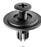
14698 (90688-SB0-003) Black Nylon Push-Type Retainer Head Diameter: 18mm Stem Length: 11mm Fits into 6mm Hole
