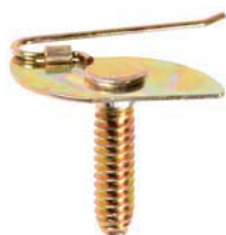
19626 (Ford: 358560; Chry: 1560058, 6010029; GM: 568792, 574355, 1165051) Moulding Fastener Bolt: #10-24 x 3/4" Plate Length: 1" Plate Width: 1/2" Replaces Auveco 2514 UNIT PACKAGE: 25
