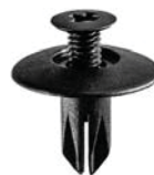
17081 (91524-SE0-003) Black Nylon Cowl Push-Type Retainer Head Diameter: 18mm Stem Length: 12mm Fits into 6mm Hole Accord 1986-On
