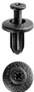
19142 (91550-SH3-003) Black Nylon Pillar Garnish, Side and Trunk Lining Push-Type Retainer Head Diameter: 15mm Stem Length: 13mm Fits into 7mm Square Hole Civic, Accord Wagon & Del Sol 1993-On
