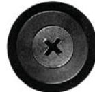
14698 (90688-SB0-003) Black Nylon Push-Type Retainer Head Diameter: 18mm Stem Length: 11mm Fits into 6mm Hole
