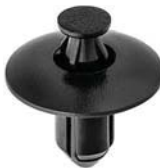
21134 (01553-09431) Black Nylon Front Bumper Push-Type Retainer Head Diameter: 20mm Stem Length: 11mm (Excluding the Pin) Fits into 8mm Hole Nissan Maxima 2004 - On
