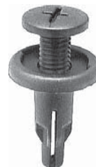
17057 (90505-SM4-003) Black Nylon Push-Type Retainer Head Diameter: 18mm Stem Length: 21mm Fits into 8mm Hole Accord 1990 - On
