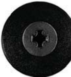
17081 (91524-SE0-003) Black Nylon Cowl Push-Type Retainer Head Diameter: 18mm Stem Length: 12mm Fits into 6mm Hole Accord 1986-On
