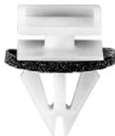
20353 (10442914) White Nylon Rocker Panel Moulding Clip Top Head Size: 1/2" x 9/16" Bottom Head Size: 9/16" x 5/8" Stem Length: 9/16" Fits into 7/16" Hole Buick Rendezvous 2002 - On
