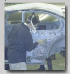
The vehicle is now ready to be painted. After painting, sanding with ultra fine grits and using various compounds and polishes can remove defects and flatten the surface, producing a better looking finish. The final sanding of the vehicle should be done using 5-1/2" x 9" waterproof 1000-1500 grit for finesse sanding of surface imperfections in enamels, acrylics or clear coats. 5-1/2" x 9" waterproof sheets are available up to 2000 grit.
