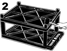
Push remaining legs onto the second shelf leg posts. Position the bottom shelf (with caster holes and ribbed design up) on top of the four legs. Once alignment is sure, again, use the rubber mallet until all four legs are seated (flush) against the surface of both the bottom and center shelves.
