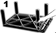
Position the center shelf with leg posts top and bottom, ribbed side up. Once alignment is sure, use the rubber mallet supplied to hammer center shelf into tubes until all four legs are seated (flush) against the surface of both the top and center shelves.
