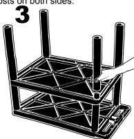
Push the four casters firmly into the holes. Make sure the two casters equipped with brakes are inserted at the same end as the operator's handle. Important: Casters must be fully seated. Tap firmly with the rubber mallet to properly seat caster. Turn your stand right side up and place your Auto Meter tester according to the operation instructions.
