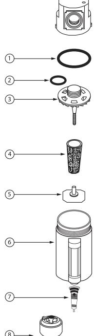
**Model 5200 Internal Float Drain Available (Item #7)** To be used for pressures from 30 psi to 175 psi and from 40°F to 120°F. To order filter with float drain assembled, add suffix "F" to filter model number.
