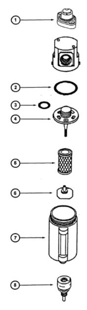
NOTE: Optional Automatic Float Drain is used for pressure from 30 psi to 175 psi, and from 40°F to 120°F
