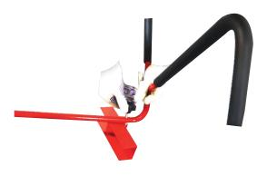
4. Affix the Work Stand Brace to the assembled Main Frame as shown above. Secure it with the Plastic Knob. Repeat instructions 1-4 for the second main frame.
