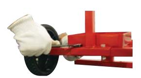
3. Attach Lower Vertical Tube to the Lower Film Holder (Base) using an M8 Bolt, Washer and Lock Nut.
