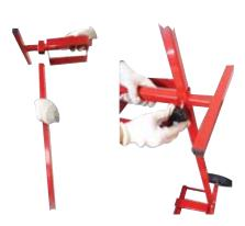
5. Slide Upper Film Holder over the Upper Vertical Tube as shown. Secure with the Knob. The Knob can be loosened so that the Upper Film Holder can slide to adjust for your film roll. Be usre to tighten the Knob after loading your film roll.
