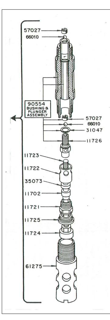
Note #2: You only remove that check ball (66010) if you suspect foreign material is behind the check ball. You can perform a visual inspection after the check ball is removed and if there is foreign debris behind the check ball, then continue and remove the bushing and plunger assembly as well. (See below).
