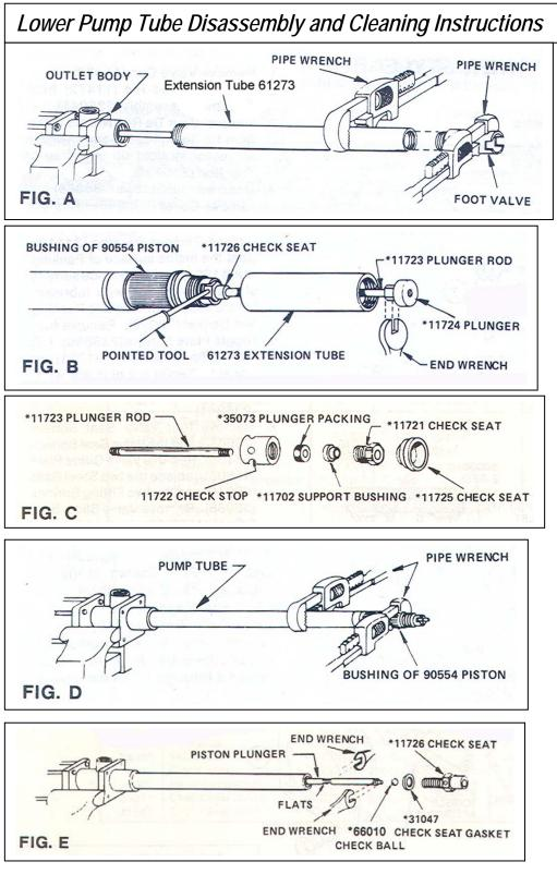
**Cleaning:** Use Mineral Spirits and a Brush to Throughly Clean all Debris out of the Foot Valve 61275 and Extension Tube 61273; Thoroughly inspect all parts for wear or damage; Clean all Parts
