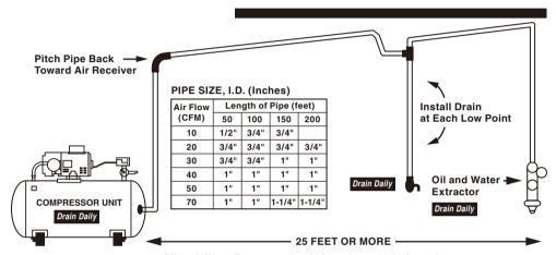
Oil and Water Extractor should be at least 25 ft. from the compressor. Further if possible.
