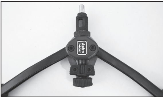
Riveter properly prepared for setting rivet nuts
